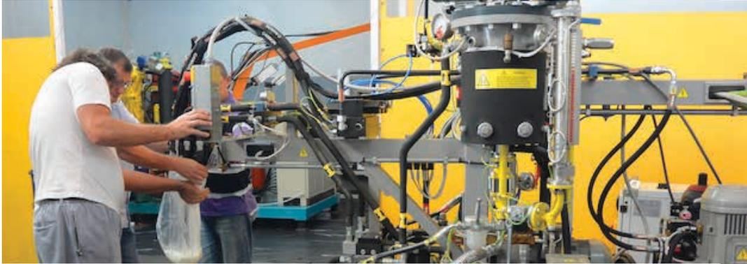
UTILISATION DE FORMIATE DE MÉTHYLE ET DE MÉTHYLAL EN REMPLACEMENT DE HCFC-141B DANS LA FABRICATION DE SEMELLES DE CHAUSSURE AU MEXIQUE. PHOTO D'HORACIO HERNANDEZ.
